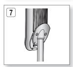
8. Insert and tighten two small screws (4x20, For connecting Stand Bracket & Speaker) into the two holes to connect them.
